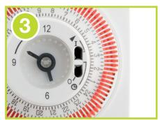
To activate the timer function, ensure that the switch on the front face is indicating the timer symbol, in the centre.
